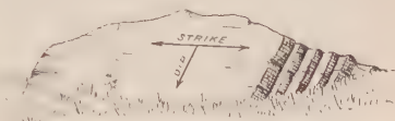
FIG. 239. — Diagram illustrating dip and strike , the dip being the angle of the greatest inclination of a bed (shown by arrow), and the strike the direction at right angles to the dip.
